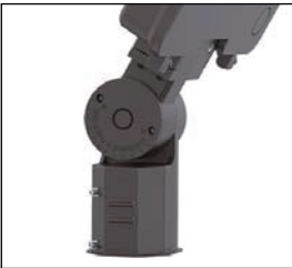
Slipfitter Mount An optional cast aluminum mast adapter secures fixture head to nominal 2-3/8" O.D. horizontal steel tenon arm.
